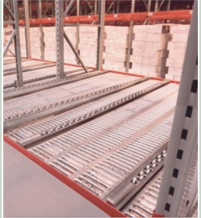
▲ Skatewheel flowrack being used for pallet picking and pallet return on the 2nd level of a pick module
