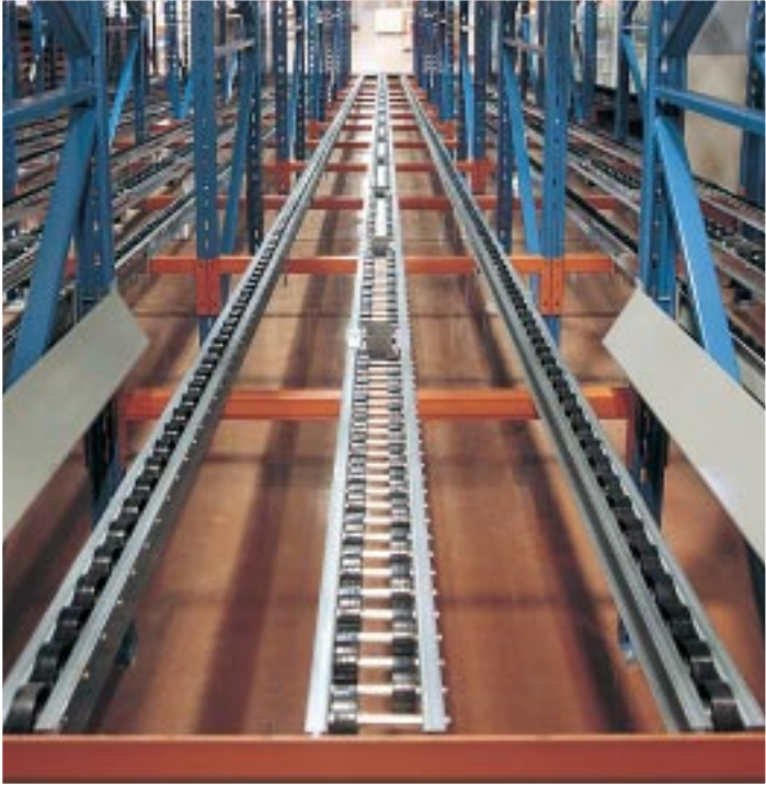
▲ Deep lane pallet flow with wheels in a single-double-single configuration for standard GMA/CHEP pallets
