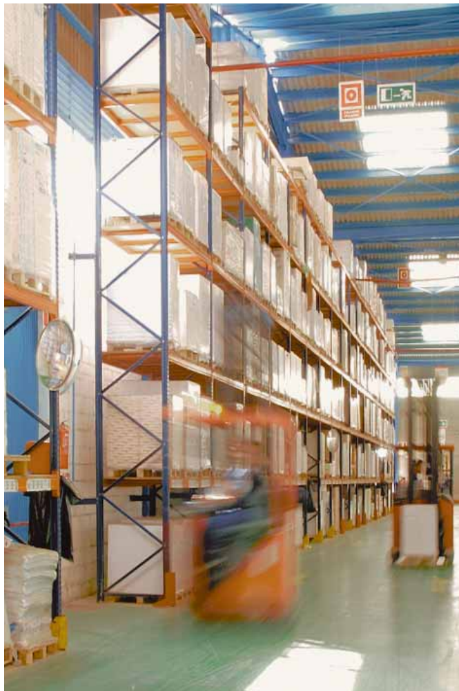
Top view of selective pallet rack warehouse. The forklift has access to rows of pallet rack on both sides.
