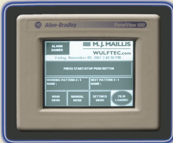
ALLEN BRADLEY AB PANELVIEW 600 IS OUR STANDARD OPERATOR INTERFACE
